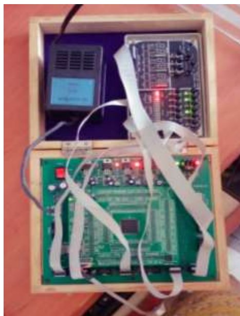
Fig.15 Implementation of Binary to gray code converter in PLA using FPGA kit.
